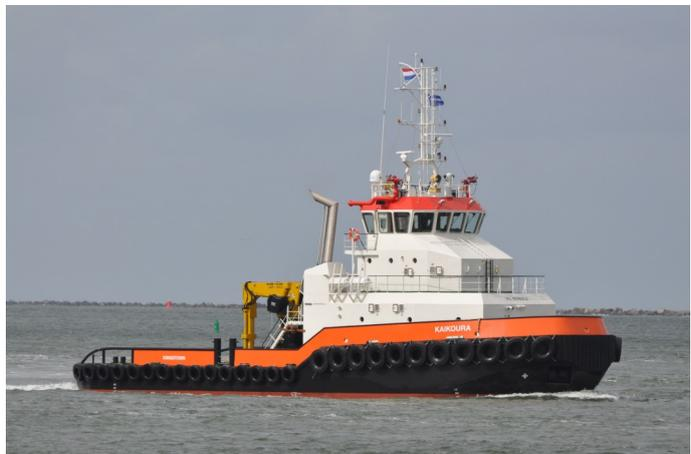
Technical specification: length overall: 35.25 mtr, beam: 11.6 mtr, draft aft: 4.22 mtr, bollard pull: 65.3 tonnes, speed: 11.6 knots.
