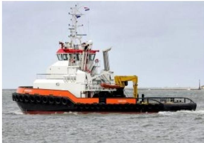
usual outfit of equipment, this new vessel has two high level fire monitors and significant pumping capacity.
